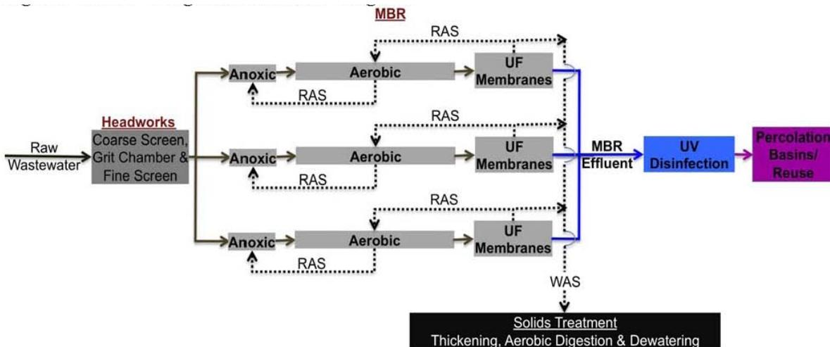
The new water recycling facility is designed to produce an effluent that meets or exceeds all current environmental wastewater quality standards mandated by the U.S. EPA and the RWQCB. The MBR is designed to produce a finished effluent with biochemical oxygen demand and total suspended solids concentrations of less than 5 milligrams per liter (mg/L), total nitrogen less than 8 mg/L and turbidity less than 0.2 Nephelometric Turbidity Units.
